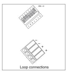
Fig 2 Terminal block connections and address 78 set
