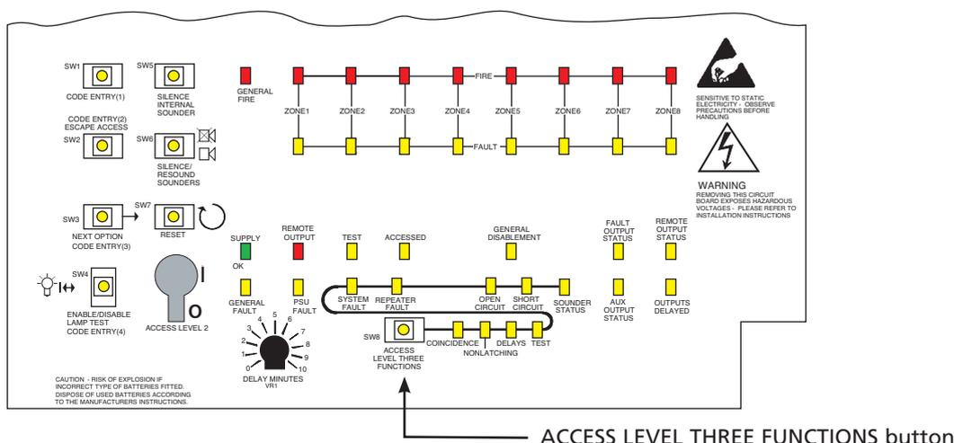
When the ACCESS LEVEL THREE FUNCTIONS button is pressed for the first time, the Accessed light will be lit steady and the first engineer function (COINCIDENCE) will be selected and indicated by its yellow light flashing (see right).
