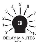
Use a small terminal screwdriver to adjust the length of the Delay period. For information on how to assign individual zones so the delay period applies to them see pages 16 and 17.
