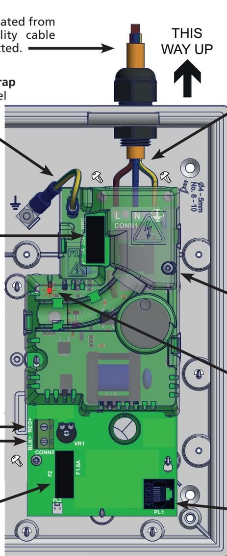
Figure 9 : Battery location and connection details
