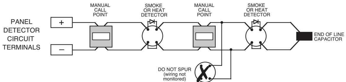
Connect an end-of-line (EOL) capacitor (provided in the panel's accessory pack) across the terminals of the last device on each circuit to allow the wiring to be monitored.
