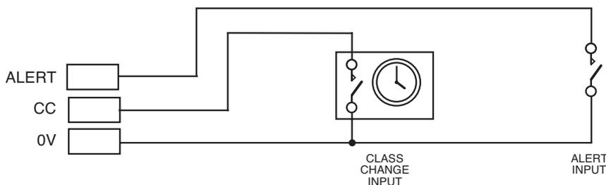
Connect the wiring for each input to the relevant 5mm connector block on the Main Control PCB and terminate their screens at the panel’s base earth distribution post (see page 13 for more details).
