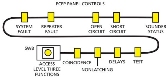
2. Continue pressing the ACCESS LEVEL THREE FUNCTIONS button until the OPEN CIRCUIT light pulses. Any existing Zone Fault lights are suppressed and the zone light(s) for any zone(s) with an open circuit fault are illuminated, e.g. if the wiring on zone 6 is broken, zone 6's Fault light will be lit.
