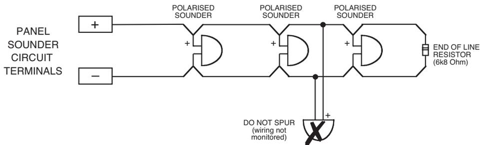
All sounders must be polarised as unpolarised sounders will show a sounder fault. A 6k8 end-of-line resistor (provided in the panel’s accessory pack) must be connected at the end of each sounder circuit to allow the wiring to be monitored.
