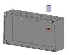
A harness is provided that extends from the battery box to the control panel. Connections are described below. You must run the harness through the knockout (removed above), through the coupling and up to the control panel battery terminal (BAT+ BAT-)
