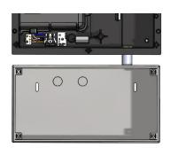
4. Attach the battery box to the coupling Using 1 x 20mm conduit bush
