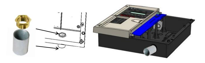
3. Remove the relevant knockout from the top of the battery box as indicated
