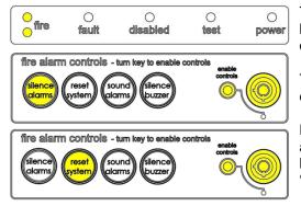
The red 'FIRE' LED will illuminate. The fire alarms and the internal buzzer will operate as programmed. Take appropriate action as defined by the emergency plan for the premises.
