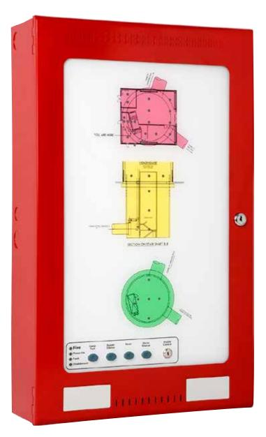
The eMatrix system uses flexible, optic light guides to illuminate areas on a floor plan, laid over a high-resolution grid. This unique system enables indicators to be moved, removed or added on site without the need for any wiring.
