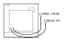
Care should be taken when terminating devices to ensure all cables are correctly sleeved and connections are secure. Improper connections will prevent a system from responding properly in the event of a fire. Please remember that all high voltage testing must be carried out before the installation of the Flashpoint front unit as this may cause damage. It is important to maintain the screen continuity in order to protect against data corruption from interference.
