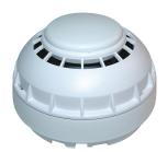
Once all testing has been carried out on the cabling and 'continuity & integrity' has been proven, the device may be assembled. To insert the Sounder unit, gently offer it into the base, rotating the device until it drops in and clicks into its locked position.
