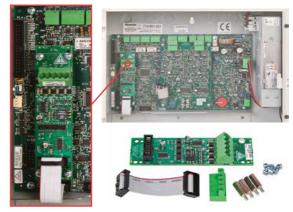
Internal view of DXc2 panel with RS232 card fitted
