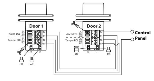
Remove jumpers J1 and J2 Cut appropriate tamper resistor link (2K2 illustrated) Connect T1 to panel
