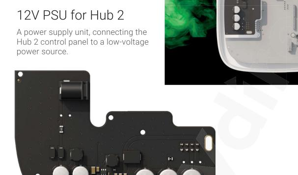
12V PSU for Hub 2 is a power supply unit, connecting the Hub 2 control panels to 12 volt DC sources. This is an electronic board, replacing the standard 110/230 V power supply unit in the body of the device.
