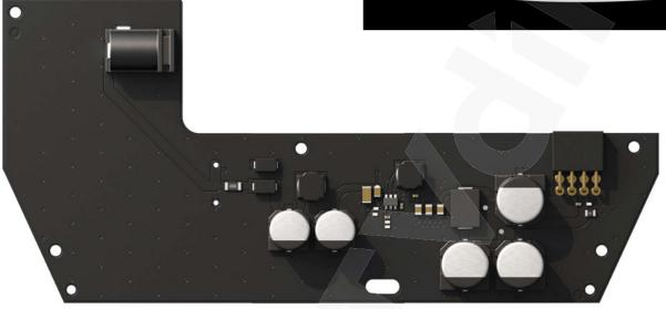
12V PSU for Hub/Hub Plus/ReX is a power supply unit, connecting the Hub/Hub Plus control panels as well as the ReX radio signal extender to 12 volt DC sources. This is an electronic board, replacing the standard 110/230 V power supply unit in the body of the device.
