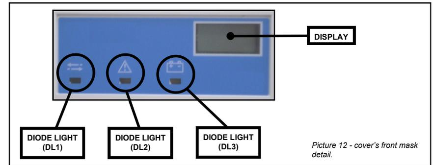
Picture 12 - cover's front mask detail.
