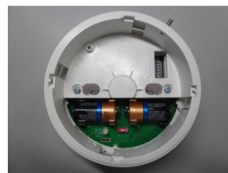
Picture 6 - primary and secondary batteries inserted
