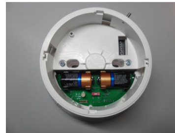
Picture 6 - primary and secondary batteries inserted
