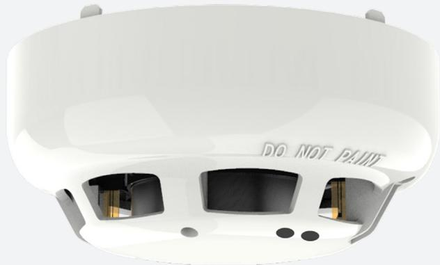
A **Multi Sensor** incorporating a thermal element and a High Performance photoelectric smoke chamber. Has three modes controlled from the Control Panel, allowing either the optical or thermal element or both to be active in making the fire decision.
