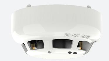
A Multi Sensor incorporating a thermal element and a High Performance photoelectric smoke chamber. Has three modes controlled from the Control Panel, allowing either the optical or thermal element or both to be active in making the fire decision.
