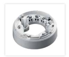
The TimeSaver Relay Base incorporates a single-pole voltage-free changeover contact for switching external equipment. When the detector changes to the alarm state, the relay is energised, causing the contact to change state. The contact will remain in this condition until the detector is reset.
