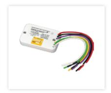
The XP95A Isolator is placed at intervals on the loop and ensures that, in the case of a short-circuit, only the section between the isolators will be affected. When the short-circuit is removed, the isolators automatically restore power and data to the isolated section.
