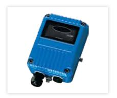
The IS IR<sup>3</sup> Flame Detector is designed for harsh environments in either indoor or outdoor applications. It is sensitive to low-frequency flickering IR radiation emitted from flames during combustion. The sensor operates even through a layer of oil, dust, water vapour or ice. These detectors have been approved by Baseefa to EN50014, EN50020 and EN50284. The requirements of Directive 94/9/EC, the Atmosphere Explosives ATEX Directive have also been met.
