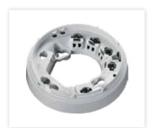
The Orbis LX Base has two slots for fixing screws at a spacing of 51mm to 69mm. Detectors fit into the base one way only and require clockwise rotation without force to be plugged in.
