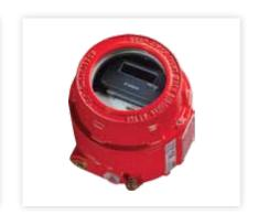
The Intelligent IR<sup>2</sup> Flame Detector is designed for harsh environments in indoor applications. The detector has two sensors which respond to different IR wavelengths to discriminate between flames and spurious sources of radiation.
