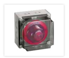
The Ceiling Tile Mounting Box has been designed to make the installation of detectors and sounders quick and easy prior to the fitting of a false ceiling. Detector and sounder bases can be fitted, wired and if necessary, tested and commissioned before the installation of a false ceiling.
