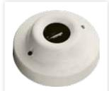
The Intelligent Base Mounted UV Flame Detector is designed to protect enclosed indoor areas where open fires may be expected. The detector has a fast acting response to flames up to 25m away and is equipped with a single UV sensor with a narrow spectral response in order to discriminate between flames and most spurious sources of radiation.
