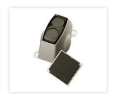
The high performance Auto-Aligning Beam Detector comprises ground level controller, detector head with auto-aligning feature, integral laser for rapid initial alignment and single prism. Up to three additional detector heads can be added to the controller.
