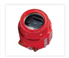
The Flameproof UV/IR² Flame Detector is designed for hazardous environments in either indoor or outdoor applications where open fires may be expected. False alarms from flickering sunlight, arc welding or lightning are avoided by the combination of UV and dual IR signal processing techniques. It detects almost all flames, including those invisible to the naked eye, e.g. hydrogen fires. Certified by ISSOP for compliance with standards EN50014, EN50018 and EN50281.
